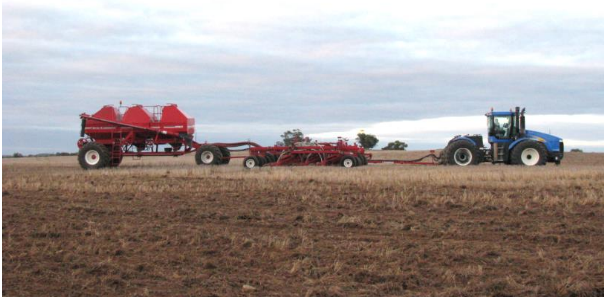
Tow-behind air-cart can add to seeder stability on the flat
