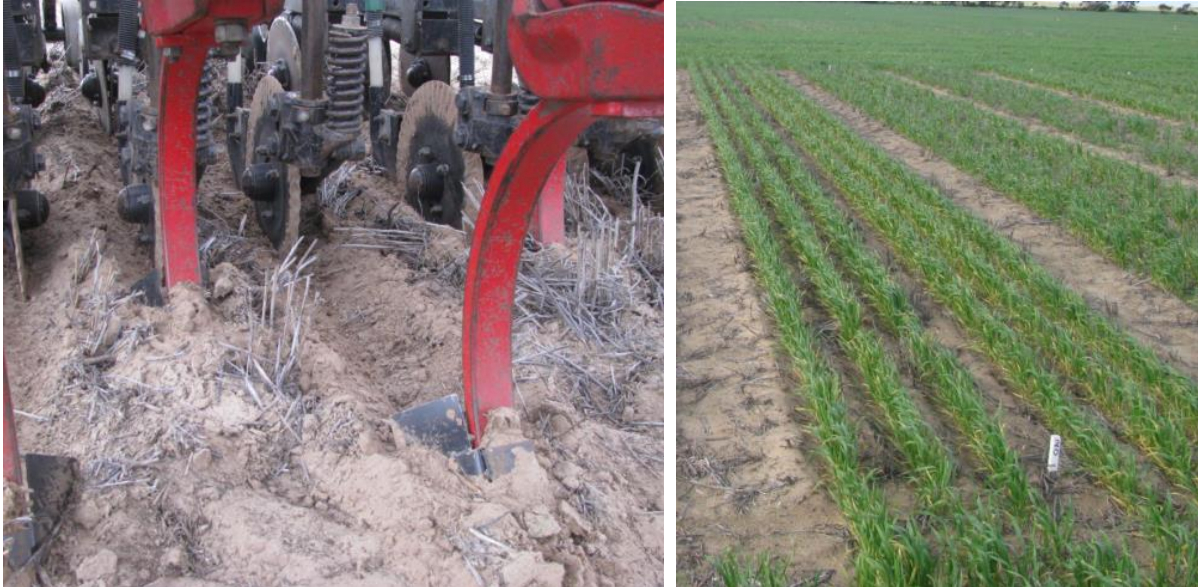
Fig. 5: Triple disc with preceding scooping share (LHS) gave the best wheat crop establishment at the 2015 Moorlands site (RHS at 71 DAS)
